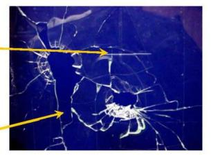
In the glass above, the top hole was made first. Notice how fracture lines from the lower penetration terminate at fracture lines from the top hole. Below: once again the top hole was penetrated first as evidenced in the close-up view.
